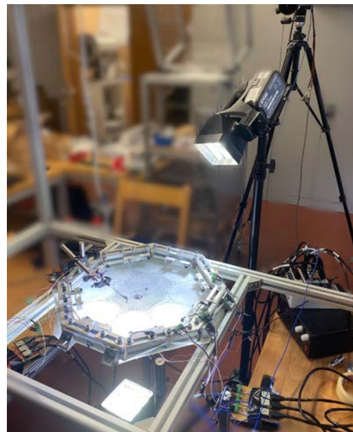
The web is suspended into an octagonal frame. Below the frame is a semi-transparent sheet. Lighting from the bottom ensures a white background, even at high frame rates. Lighting from the top ensures the web itself is sufficiently lighted at high frame rates.
