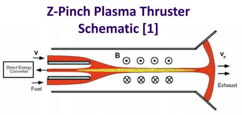
>Thermonuclear fusion occurring in the plasma creates the high energy density needed for deep space missions
