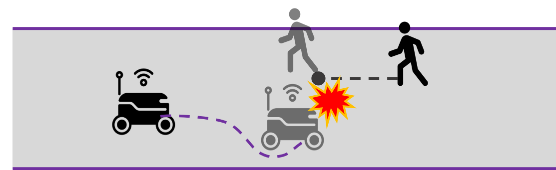
(a) Reactive planning: Illegible robot behaviors leads to collision-prone and inefficient interactions, such as the robot swerving at the last possible moment, leading to collision/near miss.
