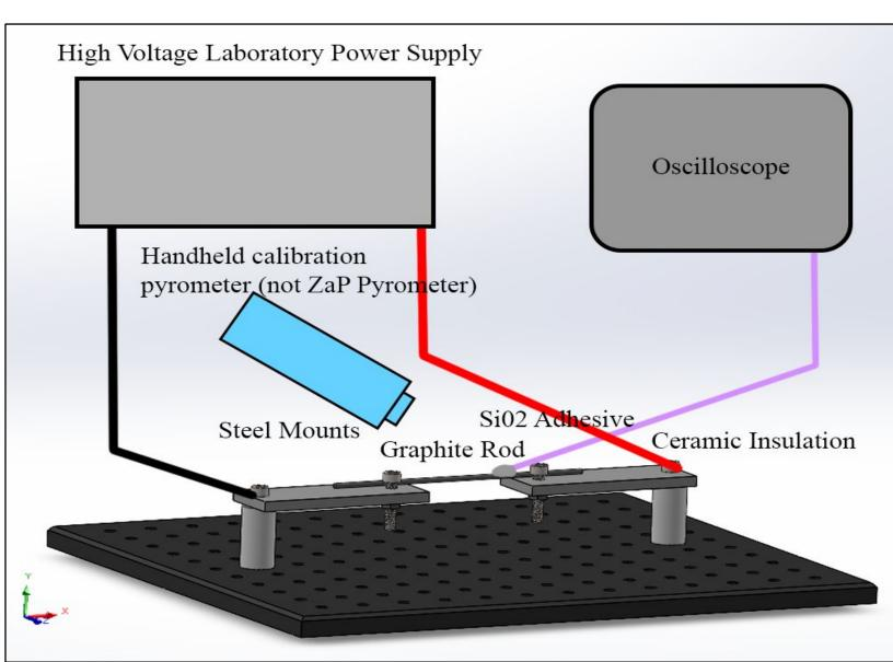
ZAP PYROMETER TARGET DIAGRAM CREDIT: ZAP LAB – WALKER HOLMQUIST
