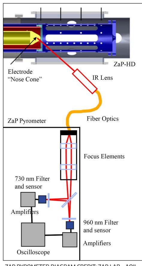
ZAP PYROMETER DIAGRAM CREDIT: ZAP LAB - AQIL
