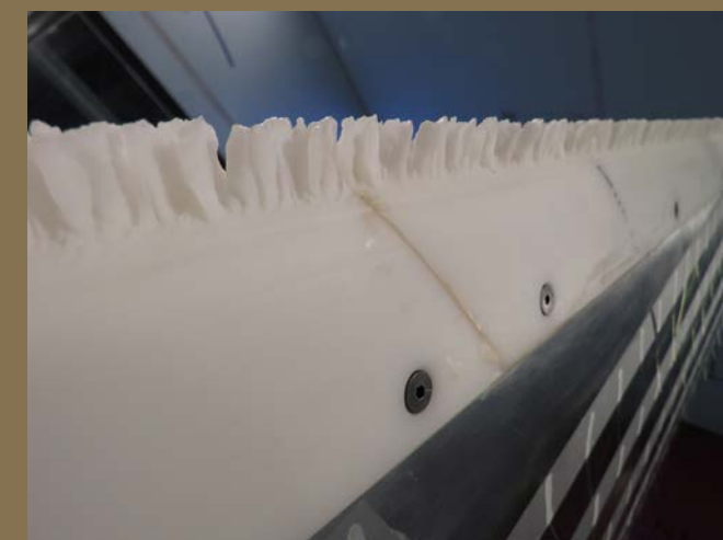
The ice accretion testing involves printing 3D CAD models of ice that NASA has developed from their own refrigerated wind tunnels. These plastic printed models can simulate the ice in non-refrigerated tunnels like the KWT. Each printed model is about 45 inches long and will be attached to the leading edge of the wing and will be fitted with 70 taps to measure pressure.
