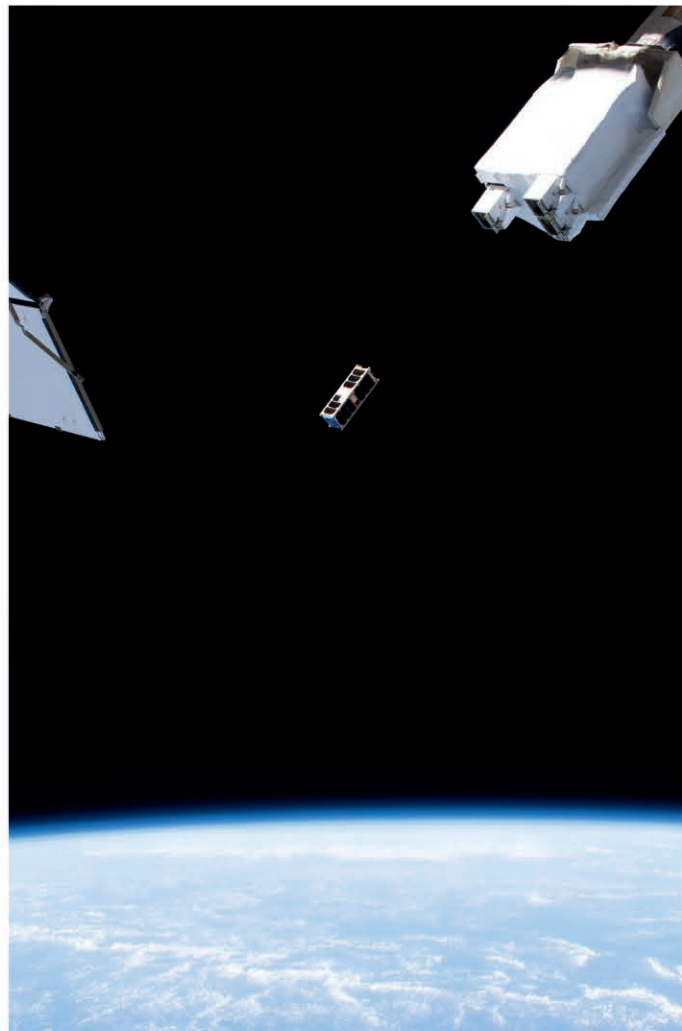
Above right: A CubeSat is deployed from the International Space Station's JEM Small Satellite Orbital Deployer. CubeSats are cheaper and lighter, therefore getting them into orbit is easier and less risky. Credits: NASA
