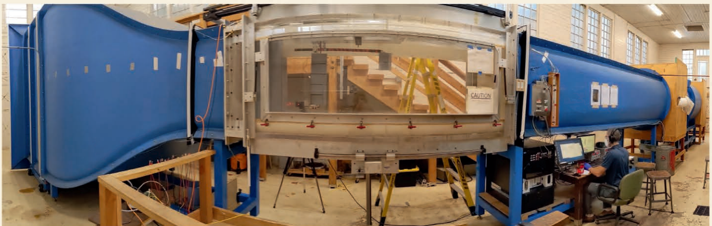
John Berg observes data on a flexible wing model installed vertically in the test section. The “3X3” serves as a good stepping stone test environment to gain initial data before moving forward in complexity and expense to the larger Kirsten Wind Tunnel. Photo by Eddie Ting.
