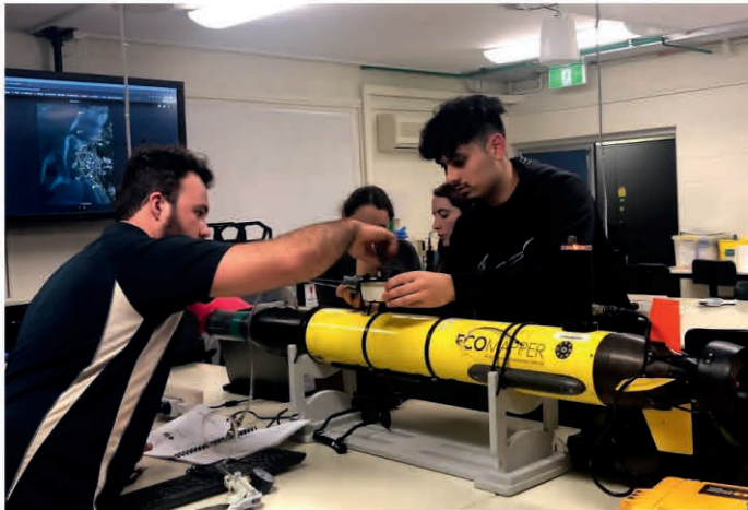
Cuadras (right) working on the autonomous underwater vehicle “Ecomapper” as part of the LSAMP summer oceanography program in Australia. The Ecomapper records salinity, pH, and more. Here, Cuadras is attaching a camera to record footage for the Ecomapper’s upcoming project to investigate seagrass beds.
